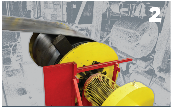
Coil is cut into sheets by our Stretcher Leveler
