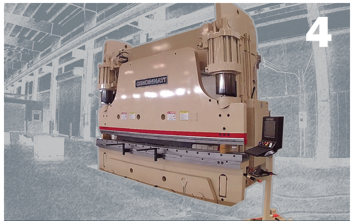
On-site press brakes bend the laser cut sheets
